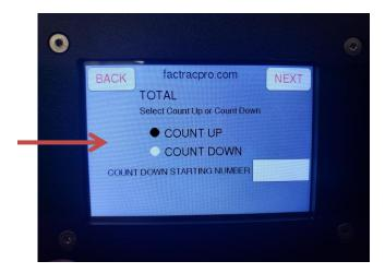
To use COUNT DOWN, press the "circle" next to Count Down. Press the number box to set the value that you want to count down from. A pop up keyboard will appear on the screen. Select the value, press the enter key. When counting down, you can assign Output 1 to activate each time the count reaches zero. Note: This count will show negative after reaching zero.
