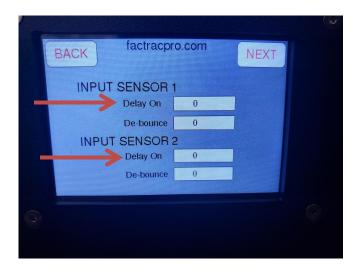
Debounce is used in cases where you may have a product that has drastic color changes or has 3D characteristics. Once the input is asserted, the count will change but then the sensor will ignore all other potential inputs for the given amount of time set for. A good setting value to start with is 5ms.
