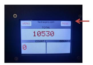
Once pressed, the Reset screen will appear and provide the options of which features you would like to reset.
