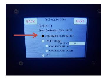
To use the Cycle Count feature, press the "circle" next to Cycle Count. You can then set the batch size to count up to or down from. When the count or zero is reached, the number displayed will reset and allow you to force an output on Output 1 or Output 2.
