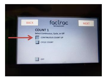
To use the Cycle Count feature, press the "box" next to Cycle Count. You can then set the batch size to count up to or down from. When the count or zero is reached, the number displayed will reset and allow you to force an output on Output 1 or Output 2.
