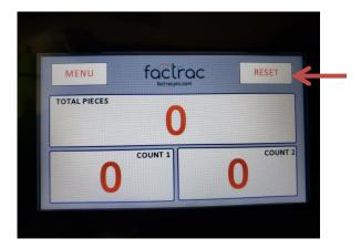
Once pressed, the Reset screen will appear and provide the options of which features you would like to reset. Any time one of the Reset buttons is pressed, you will receive a pop up to confirm. Simply touch Yes or Cancel to proceed. Then press the Back button to return to the Home Screen.
