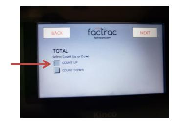
To use COUNT DOWN, press the "box" next to Count Down. Press the number box to set the value that you want to count down from. A pop up keyboard will appear on the screen. Select the value, press the enter key, and then press the SET button. When counting down, you can assign Output 1 to activate each time the count reaches zero. Note: This count will show negative after reaching zero.
