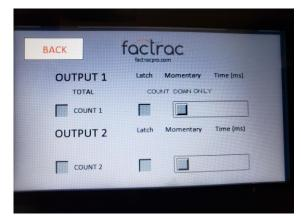
To latch the output, press the "box" below Latch. Based on your other settings, when the value reaches its target, the output will latch and remain until Reset is pressed.
