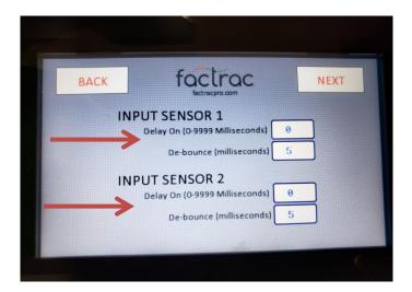
Debounce is used in cases where you may have a product that has drastic color changes or has 3D characteristics. Once the input is asserted, the count will change but then the sensor will ignore all other potential inputs for the given amount of time set for. A good setting value to start with is 5ms.
