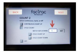
Next, you can assign Count 1 to Cycle Count Up or Down by pressing the "box" next to the desired one. Cycle Count Up will start at zero. Once the batch size is reached, it will reset to zero. Cycle Count Down will start at the number you entered in for the Batch Size. Once the count reaches zero, it will reset to the beginning number.
